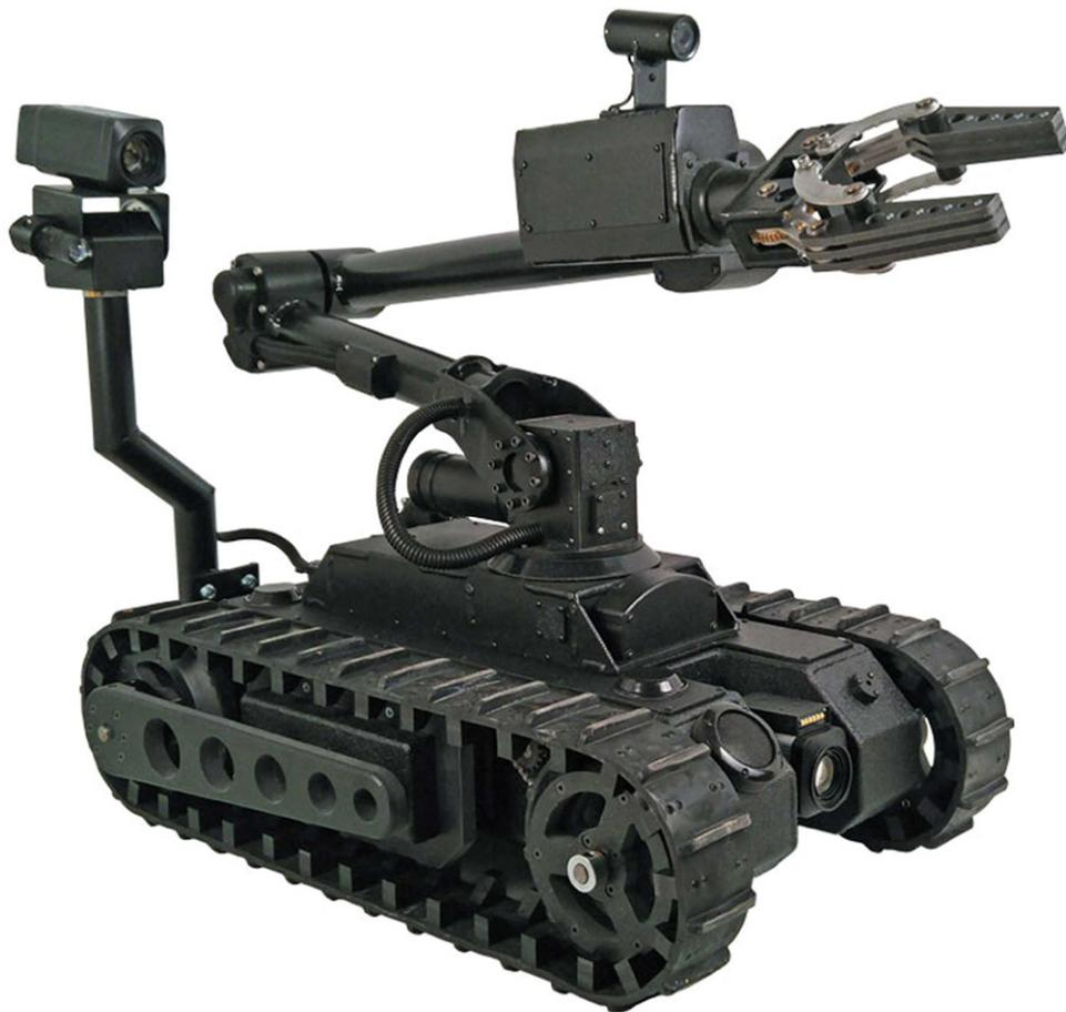
The SuperDroid Robots LT2-FTZPTZA-526 Surveillance Robot with a removable 6-Axis arm is a medium sized, rugged robot that can be quickly deployed in an emergency.
